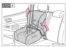
While pushing the child seat into the seat, allow the shoulder belt to retract until the child seat is securely in place.
