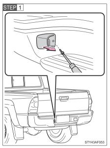
Remove the screw and light unit.
