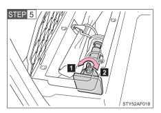
Loosen and remove the jack.
