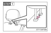
Push a flathead screwdriver into the slot. The slot is located on the left side of the right head restraint anchor.
