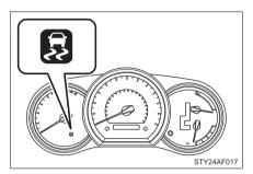
If the vehicle is in danger of slipping or rolling backward when starting on an incline, or if any of the drive wheels spins, the slip indicator light flashes to indicate that the VSC/Trailer Sway Control/TRAC/hill-start assist control systems are operating.
