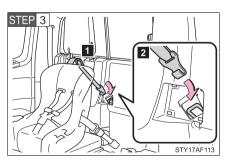
■ Route the top tether strap through the routing device as shown in the illustration.
