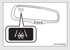
If the outside temperature lowers to 37°F (3°C) or below when the engine switch is in the ON position, the indicator will come on to warn the driver that roads may be icy. Check the road surface and drive carefully. (The indicator will go off when the outside temperature rises to 41°F [5°C].)
