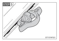
Check the tie-down cleat to confirm that it is locked into a detent and securely mounted to the deck rail system.
