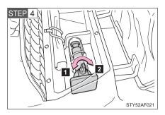
Loosen and remove the jack.
