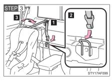
■ Route the top tether strap through the routing device as shown in the illustration.
