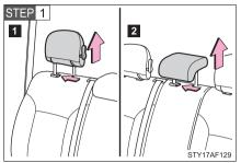
Remove the head restraint.
