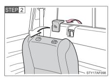
Swing the seatback forward slightly (→P. 50) and remove the anchor bracket cover.
