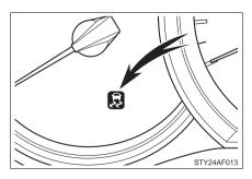
If the rear wheels spin, the slip indicator flashes to indicate that the AUTO LSD system has been controlled the spinning of the rear wheels.
