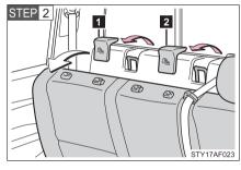
Swing the seatback forward slightly (→P. 50) and remove the anchor bracket covers.
