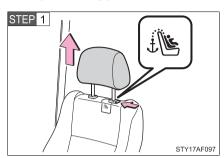
Remove the head restraint.
