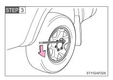
Slightly loosen the wheel nuts (one turn).
