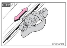
Slide the cleat to the closest detent in the rail system. You will feel that the locking plate snaps into a detent.
