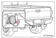
Use the wire harness stored in the rear end under the vehicle body.
