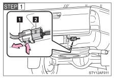
To disconnect the wire harness connectors (1 and 2), press and hold the lock of the tailgate wire harness connector (White) and pull apart.
