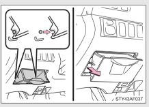
2.Pull up the box and disengage the claws. Remove the stoppers from the cutouts and remove the box. STEP 3 After a system failure, see "Fuse layout and amperage ratings" (→P. 477) for details about which fuse to check.
