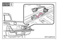
Pull out the wire harness from the vehicle bed.
