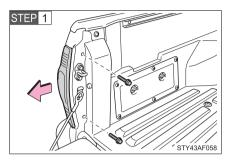
Remove the bolts and rear combination assembly.
