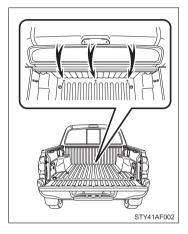
Clean the drainage hole of the deck regularly.
