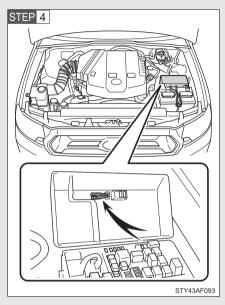
Remove the fuse with the pullout tool.
