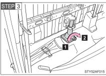
Loosen and remove the jack.
