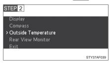
Type A: Press <u>&</u> and select "Outside Temperature", then press and hold <u>&</u>.
