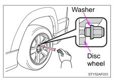
Tighten the nuts until the washer of the nut comes into loose contact with the disc wheel.
