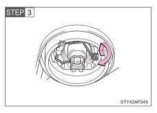
Release the bulb retaining spring.
